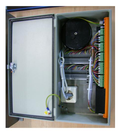
The switch board does have all the electronic equipment for the swing door drive unit C90 Su included. The distance from the switch board to the drive can not exceed more then 30 meters and should be mounted as close as possible near the drive unit also in order to keep the size of the wires small.
